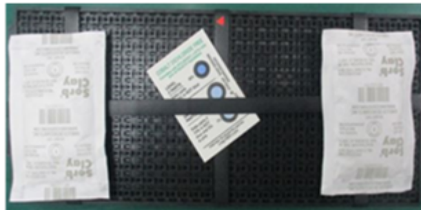
Figure 15: Tray bundle (5 loaded trays + 1 cover) with desiccant and humidity card
