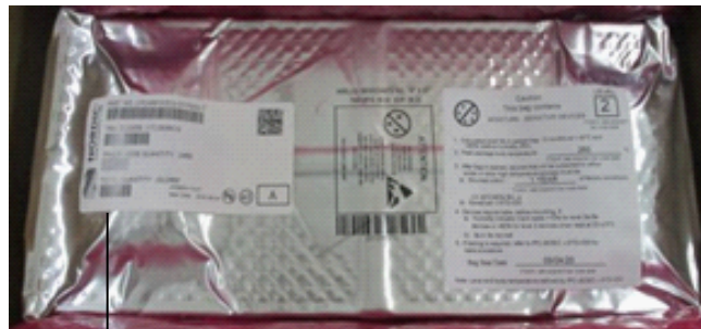
Figure 15: Tray bundle (5 loaded trays + 1 cover) with desiccant and humidity card
