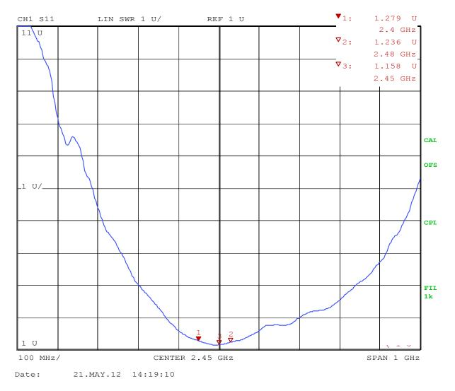
Figure 41 SWR after matching option (b)
