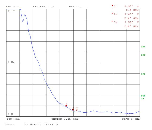
*Figure 39 SWR after matching option (a)*
