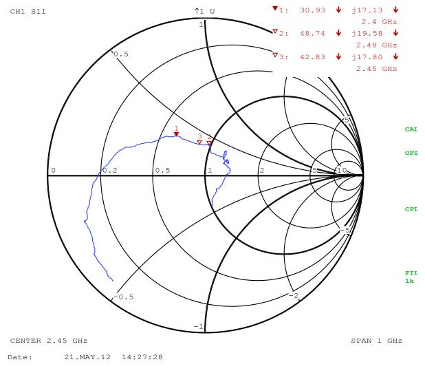
*Figure 38* Impedance after matching option (a)
