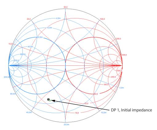
Figure 20 Adding more than one component, initial impedance
