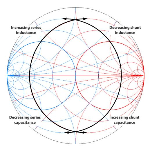
*Figure 4 Moving the impedance point*
