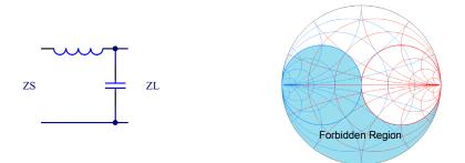
Figure 14 Network configuration with corresponding forbidden region
