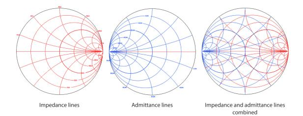
*Figure 5* Impedance and admittance lines
