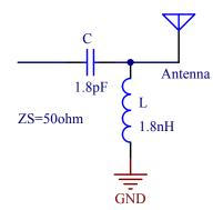
*Figure 23 Pi network configuration*
