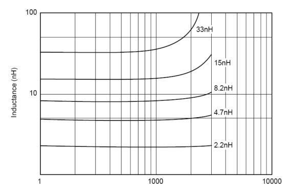
*Figure 26 Inductor values over frequency*
