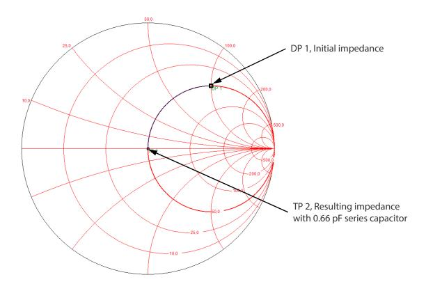
Figure 18 Adding a series capacitor
