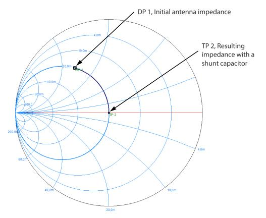
Figure 6 Shunt capacitor
