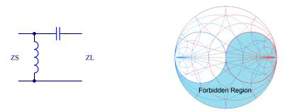
Figure 13 Network configuration with corresponding forbidden region
