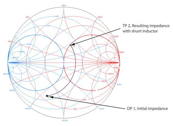
Figure 21 Adding more than one component, first step: shunt inductor added
