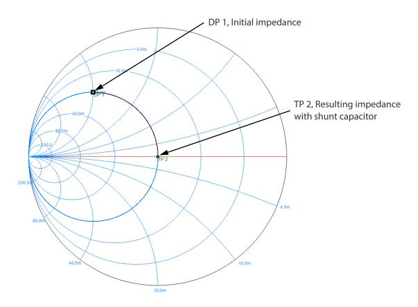
*Figure 19 Adding a shunt capacitor*
