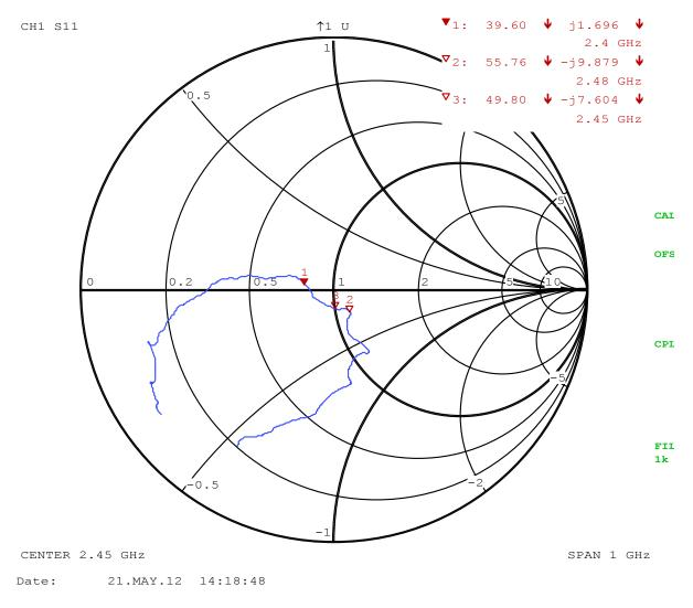
*Figure 40* Impedance after matching option (b)
