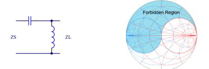
Figure 15 Network configuration with corresponding forbidden region
