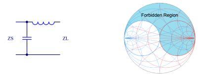
Figure 16 Network configuration with corresponding forbidden region
