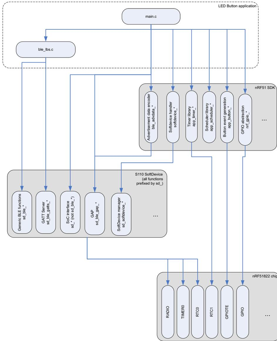
**Figure 3** LED Button application interfaces with the nRF51 SDK, S110 SoftDevice, and nRF51822 chip
