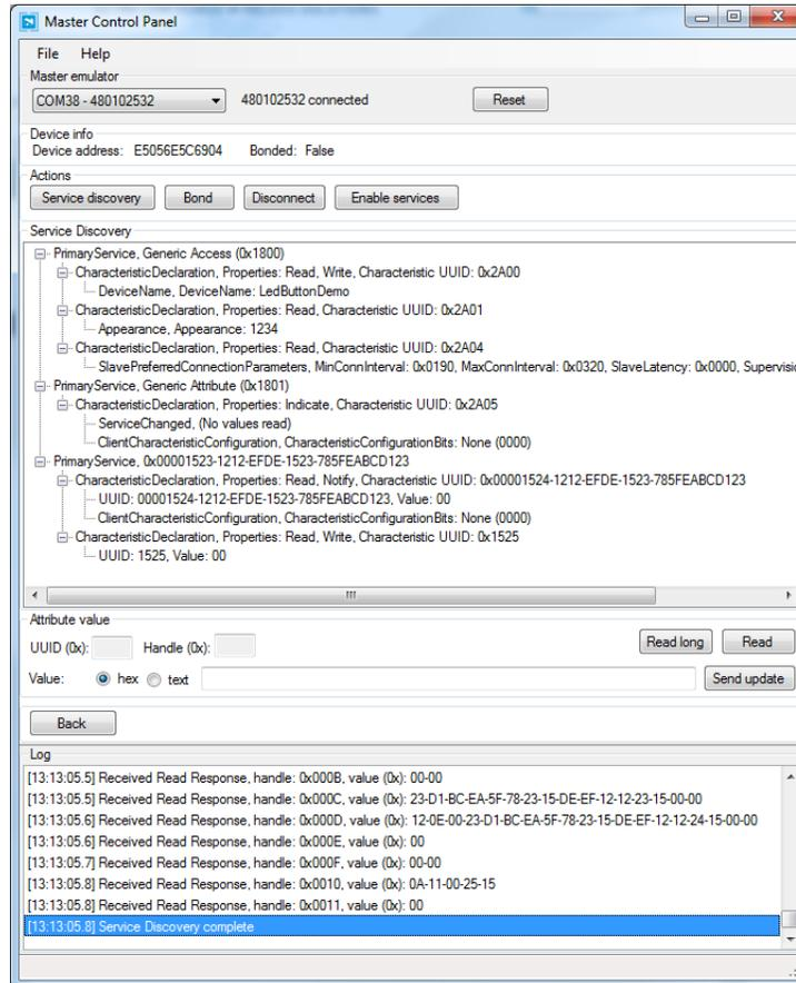
**Figure 9** Master Control Panel after service discovery
