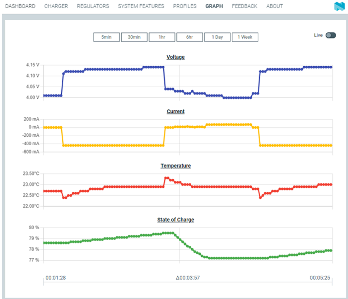
Figure 2: Evaluating the battery model in nPM PowerUP
