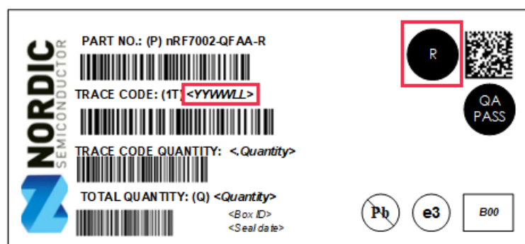
Figure 1: Trace code and black R sticker on nRF7002 label
