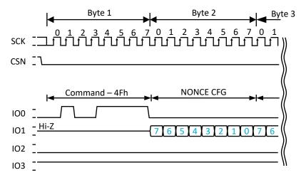
Figure 7: CIPHER INIT (Initialize cipher)
