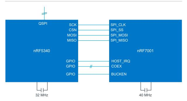
Figure 22: SPI connection
