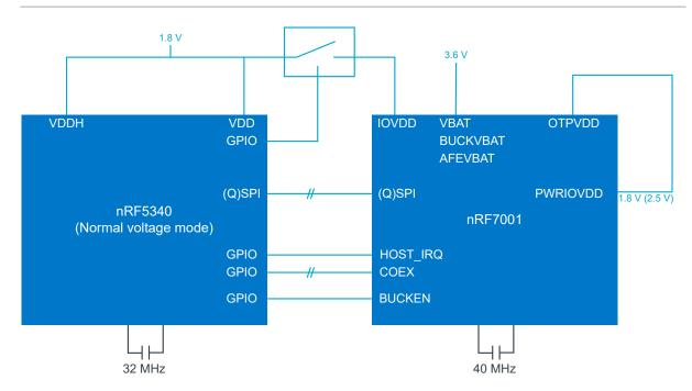
Figure 20: Supply system - normal voltage mode
