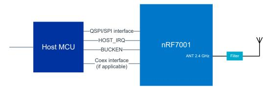
Figure 2: Functional block diagram with generic host MCU
