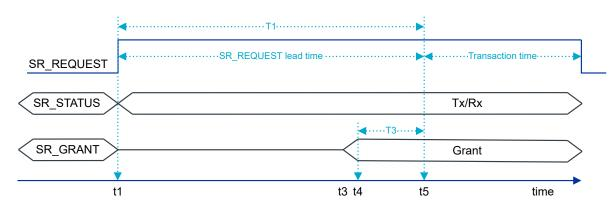
Figure 15: 3-wire timing without priority multiplexing
