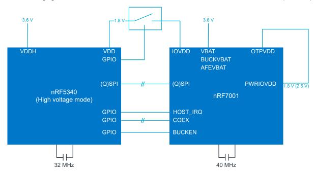
Figure 19: Supply system - high voltage mode
