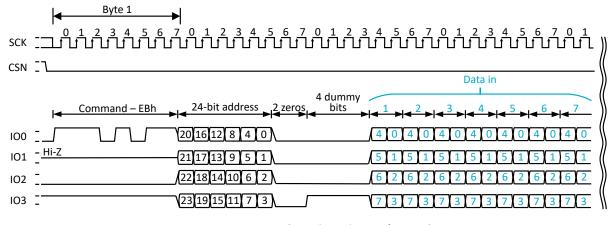
Figure 9: READ4IO (Quad-read input/output)
