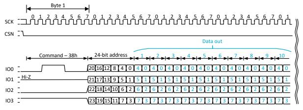
Figure 11: PP4IO (Quad-page program input/output)
