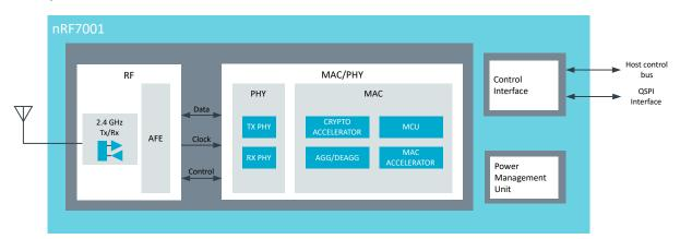
Figure 1: nRF7001 block diagram
