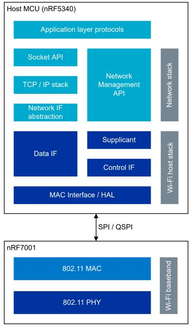
Figure 5: Network stack architecture
