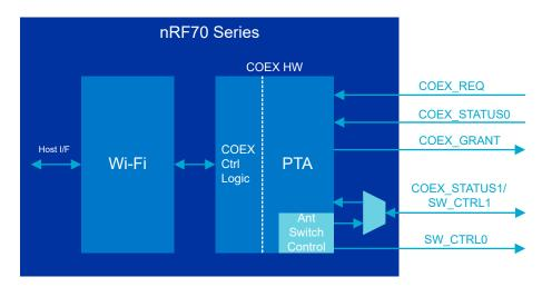
Figure 13: Coexistence hardware architecture
