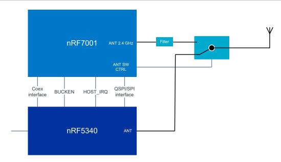
Figure 4: Functional block diagram of nRF7001 with nRF host and single antenna
