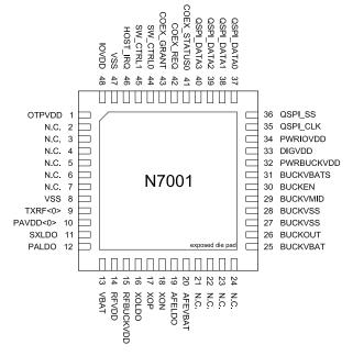
Figure 17: Pin assignments
