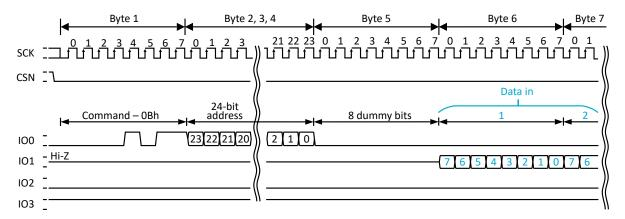
Figure 8: FASTREAD (Read bytes at higher speed)
