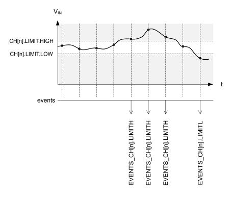
Figure 96: Example of limits monitoring on channel 'n'
