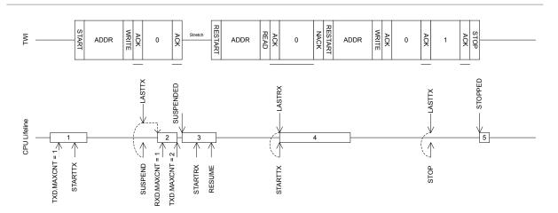
*Figure 120: A double repeated start sequence using the SUSPEND task to secure safe operation in low priority interrupts*
