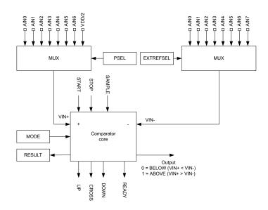
Figure 34: Comparator in differential mode
