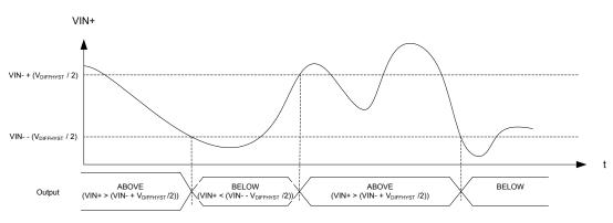
Figure 35: Hysteresis enabled in differential mode
