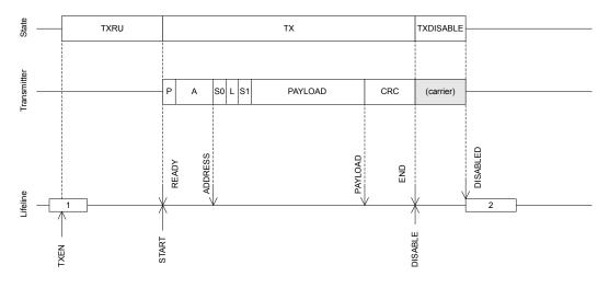
Figure 64: Transmit sequence using shortcuts to avoid delays
