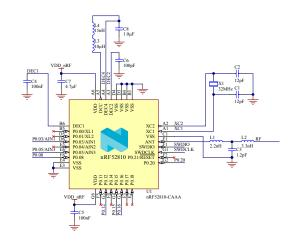
Figure 149: CAAA WLCSP 2-layer setup
