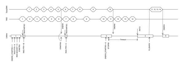
Figure 136: UARTE reception with forced stop via STOPRX
