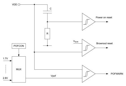
Figure 15: Power supply supervisor
