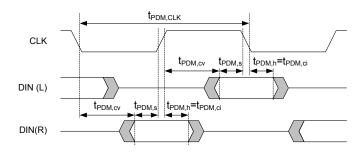
Figure 45: PDM timing diagram
