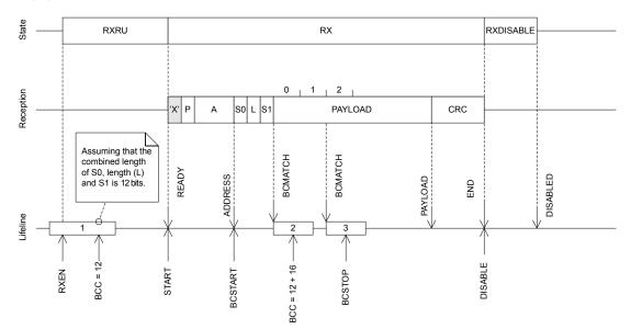
Figure 70: Bit counter example
