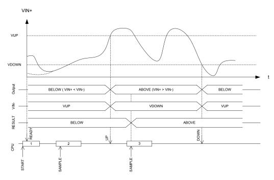
Figure 37: Hysteresis example where VIN+ starts below VUP
