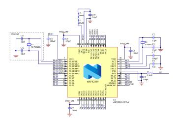
Figure 144: QFAA QFN48 with DC/DC regulator setup
