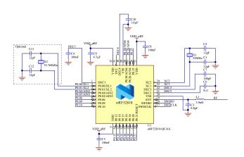
Figure 145: QCAA QFN32 with internal LDO regulator setup
