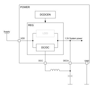
Figure 14: DC/DC regulator setup
