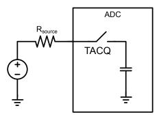
Figure 95: Simplified ADC sample network
