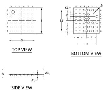
Figure 142: WLCSP 2.482 x 2.464 mm package
