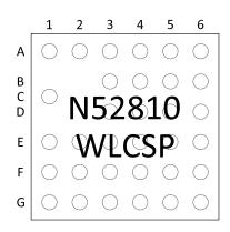
Figure 139: WLCSP ball assignments, top view
