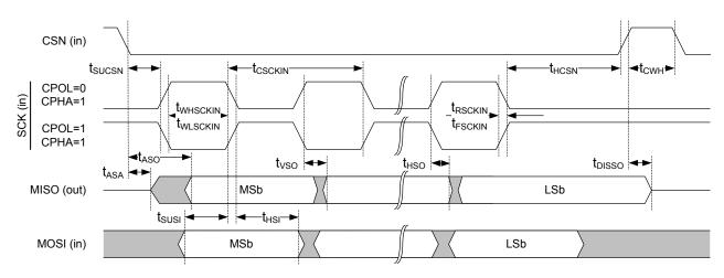
Figure 106: SPIS timing diagram
