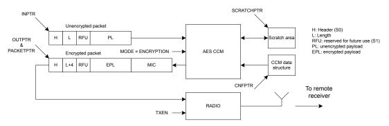
Figure 29: Configuration of on-the-fly encryption
