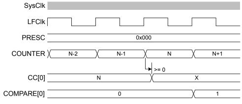
Figure 84: Timing diagram - COMPARE\_N-1
