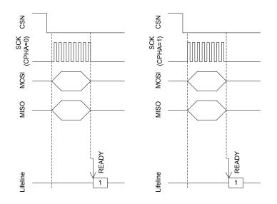
Figure 99: SPI master transaction
