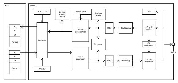
Figure 57: RADIO block diagram
