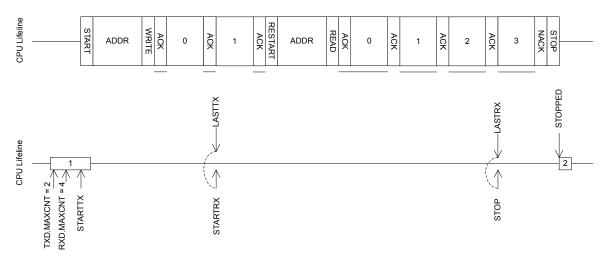
Figure 119: A repeated start sequence, where the TWI master writes two bytes followed by reading 4 bytes from the slave
