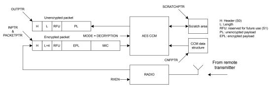
Figure 31: Configuration of on-the-fly decryption
