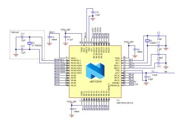
Figure 143: QFAA QFN48 with internal LDO regulator setup
