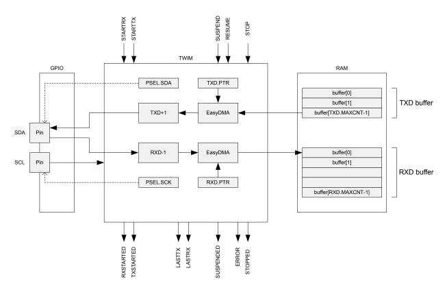
Figure 115: TWI master with EasyDMA
