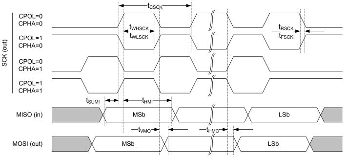
Figure 100: SPI master timing diagram
