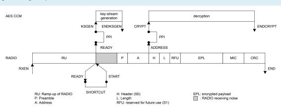
*Figure 32: On-the-fly decryption of short packets (MODE.LENGTH = Default) using a PPI connection*
