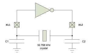
Figure 20: Circuit diagram of the 32.768 kHz crystal oscillator
