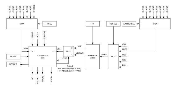
Figure 36: Comparator in single-ended mode
