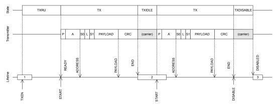
Figure 65: Transmission of multiple packets
