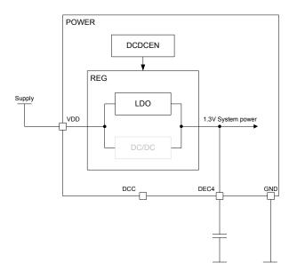
Figure 13: LDO regulator setup
