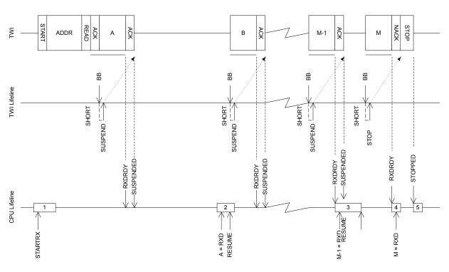
Figure 111: The TWI master reading data from a slave
