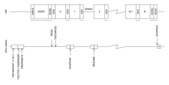
*Figure 126: The TWI slave responding to a read command*
