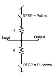
*Figure 94: Resistor ladder for positive input (negative input is equivalent, using RESN instead of RESP)*
