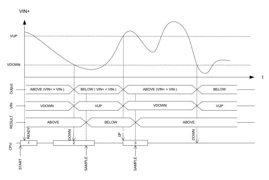
Figure 38: Hysteresis example where VIN+ starts above VUP
