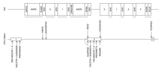
*Figure 128: A repeated start sequence, where the TWI master writes two bytes followed by reading four bytes from the slave*
