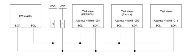
Figure 109: A typical TWI setup comprising one master and three slaves
