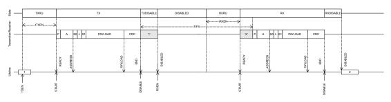
Figure 69: Ramp up and TIFS Timing Details
