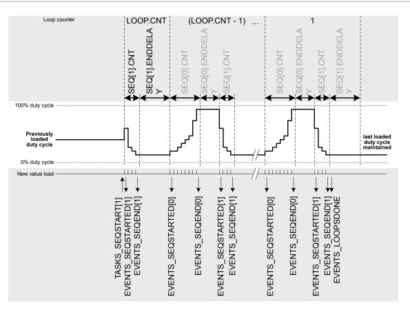
Figure 55: Complex sequence (LOOP.CNT>0) starting with SEQ[1]
