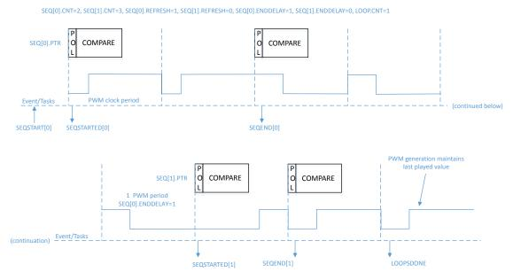
Figure 52: Example using two sequences
