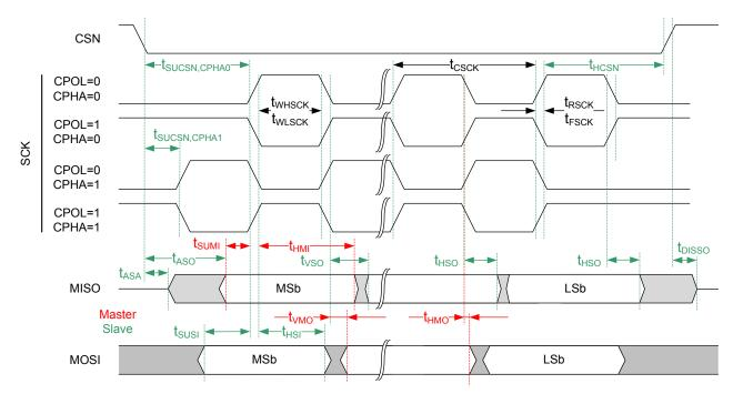
Figure 107: Common SPIM and SPIS timing diagram
