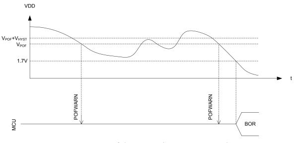
Figure 16: Power-fail comparator (BOR = Brownout reset)
