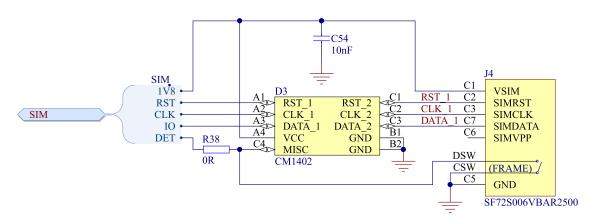
Figure 10: SIM card schematic
