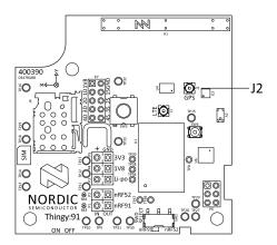
Figure 8: External GPS antenna connector
