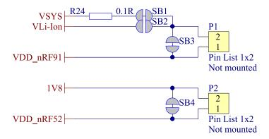
Figure 24: Current measurement schematic
