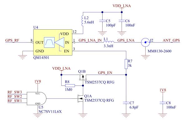
Figure 9: GPS circuit schematic
