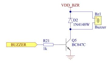
Figure 17: Buzzer schematic
