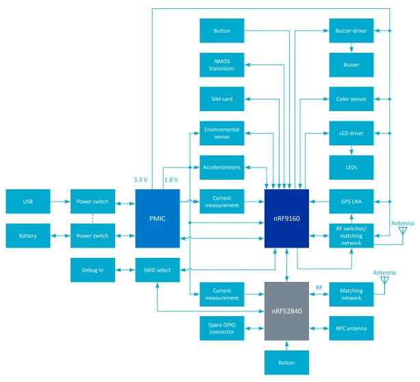
Figure 2: Nordic Thingy:91 hardware block diagram
