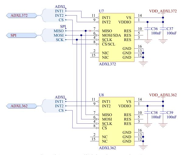
Figure 13: Low-power and high-G accelerometers schematic
