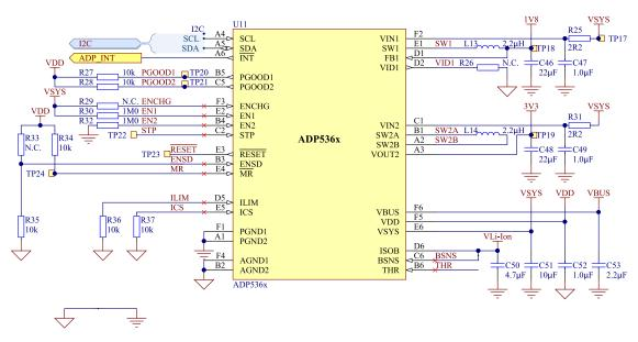
Figure 21: PMIC schematic
