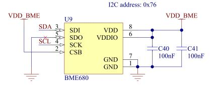
Figure 15: Environment sensor schematic
