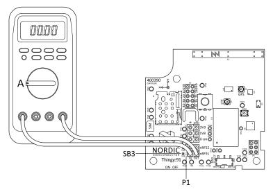
Figure 22: Measuring current to the nRF9160
