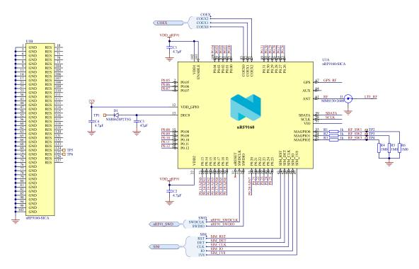
Figure 5: nRF9160 schematic
