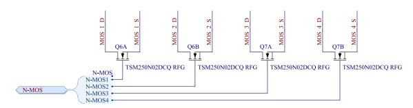
Figure 27: Schematics for the N-MOS transistors
