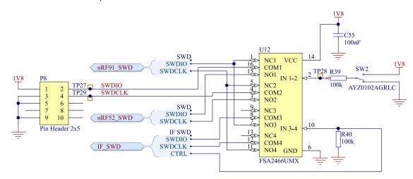
Figure 26: SWD interface and control schematic
