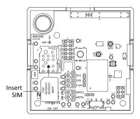
**4.** Once the *SIM* card is inserted, power on Nordic Thingy:91. You will find the power switch next to the micro-USB port.
