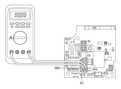
Figure 23: Measuring current to the nRF52840
