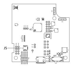
Figure 12: NFC antenna connector
