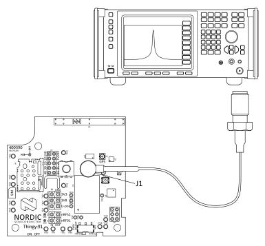
Figure 7: Connecting a spectrum analyzer
