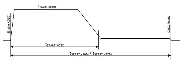
Figure 7 Current drawn at oscillator startup
