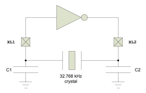
Figure 6 Circuit diagram of the 32.768 kHz crystal oscillator
