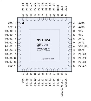
Figure 2 Pin assignment - QFN48 packet
