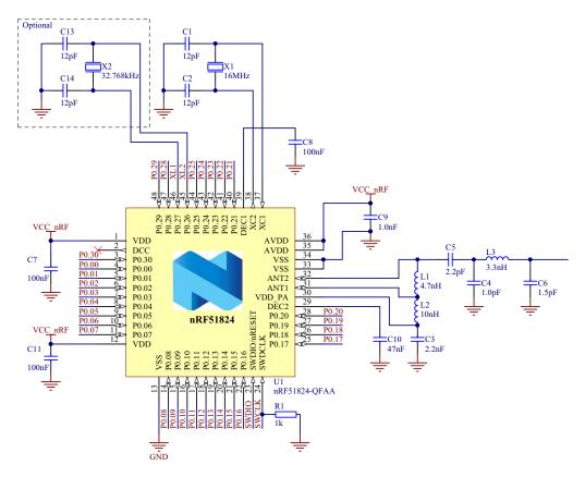
Figure 16 QFAA QFN48 with internal LDO setup
