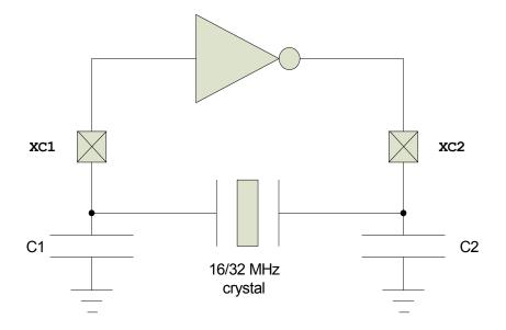
Figure 5 Circuit diagram of the 16/32 MHz crystal oscillator
