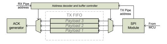
Figure 10. TX FIFO (PRX) with pending payloads
