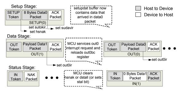
Figure 29. Control Write Transfer
