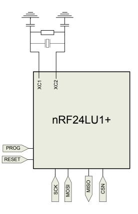
Figure 68. Clock source from a crystal between XC1 and XC2 pins
