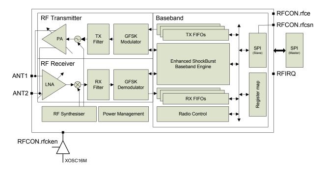
Figure 4. RF Transceiver block diagram
