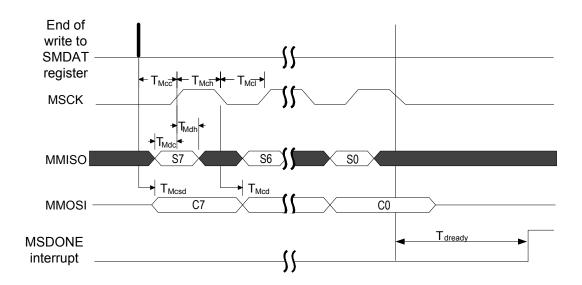
Figure 47. Master SPI timing
