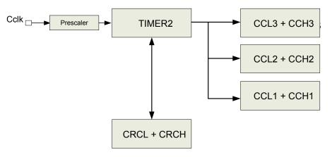
Figure 56. Timer 2 block diagram
