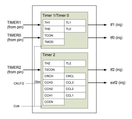
Figure 50. Block diagram of timers/counters
