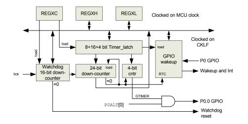
Figure 72. Block diagram of wakeup and watchdog functions
