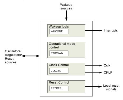
Figure 73. Power management block diagram
