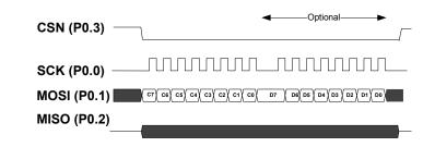
Figure 65. SPI write command without address
