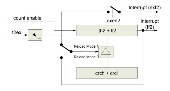
Figure 57. Timer 2 in Reload Mode
