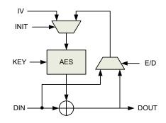
Figure 43. CFB – Cipher FeedBack mode
