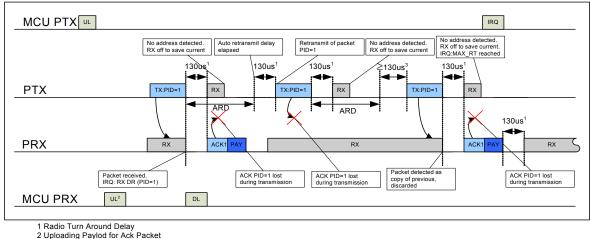
2 Uploading Paylod for Ack Packet 3 Delay defined by MCU on PTX side,  $\geq$  130us
