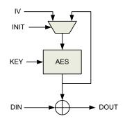
Figure 44. OFB – Output FeedBack mode
