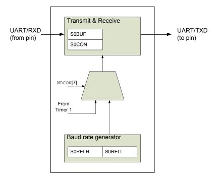
Figure 58. Block diagram of serial port
