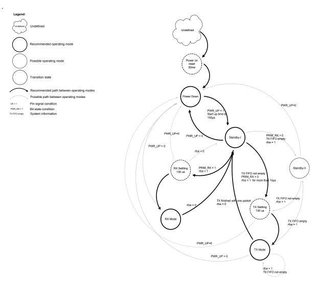
Figure 5. Radio control state diagram
