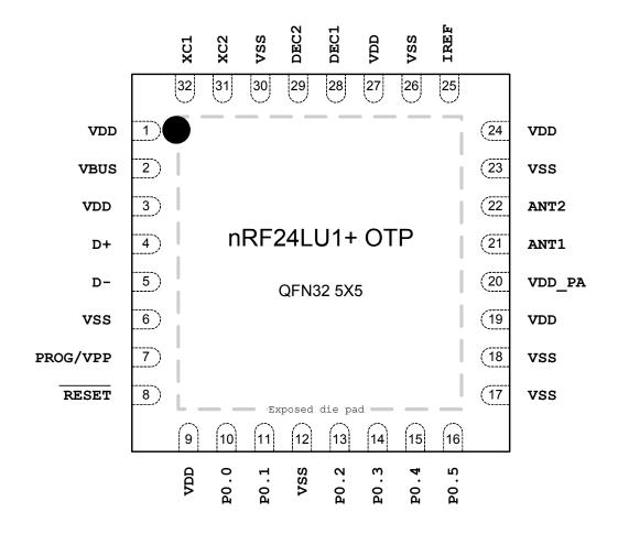
Figure 3. nRF24LU1+ OTP pin assignment (top view) for a QFN32 5x5 mm package.
