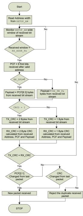
Figure 9. Automatic packet disassembly
