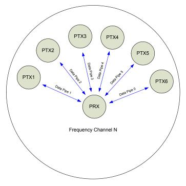
Figure 13. PRX using MultiCeiver™
