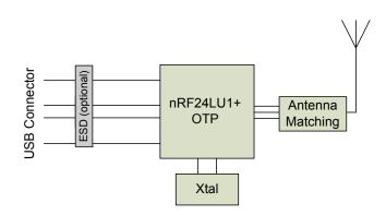
Figure 2. Typical system usage
