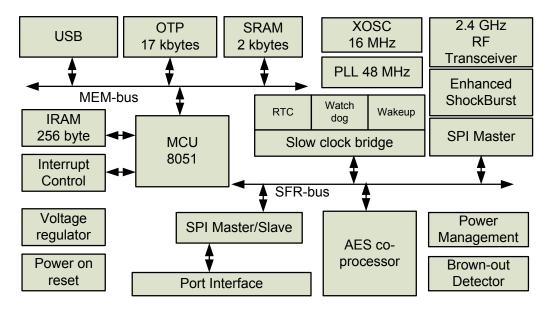
Figure 1. nRF24LU1+ OTP block diagram
