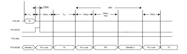
Figure 18. Timing of Enhanced ShockBurst<sup>™</sup> when the first ACK packet is lost (2Mbps)
