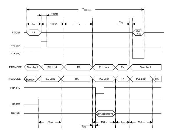
Figure 17. Timing of Enhanced ShockBurst<sup>™</sup> for one packet upload (2Mbps)
