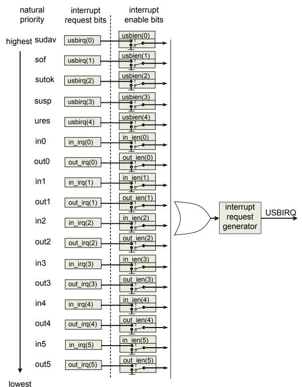
Figure 40. The USB controller interrupt sources
