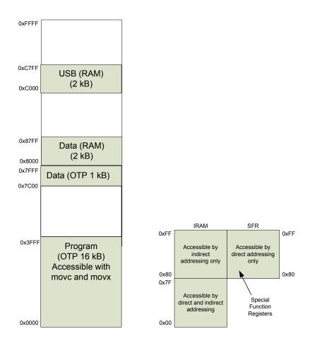
**Note:** In a program running in a protected OTP area, movc may not be used to access addresses 0x00 to 0x03.
