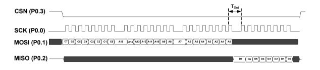
Figure 64. SPI OTP read operation, shown with 1 databyte
