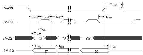
Figure 49. Slave SPI timing diagram
