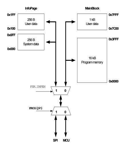
Note: The PROG pin has logical has logical level "1" at 3.3V and 6.75V. Logical level "0" at 0V.
